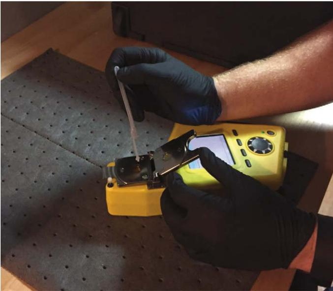
*An oil sample is inserted into the FluidScan for analysis. (Photo: U.S. Coast Guard)*
