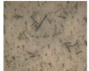
**Fatigue wear particles**
