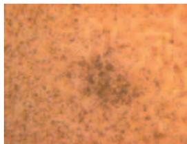
**Corrosive wear particles**
