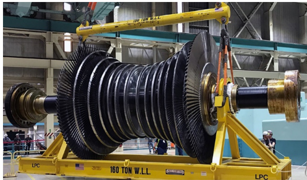
Figure 2: One compression stage from an 800 MW steam turbine.
