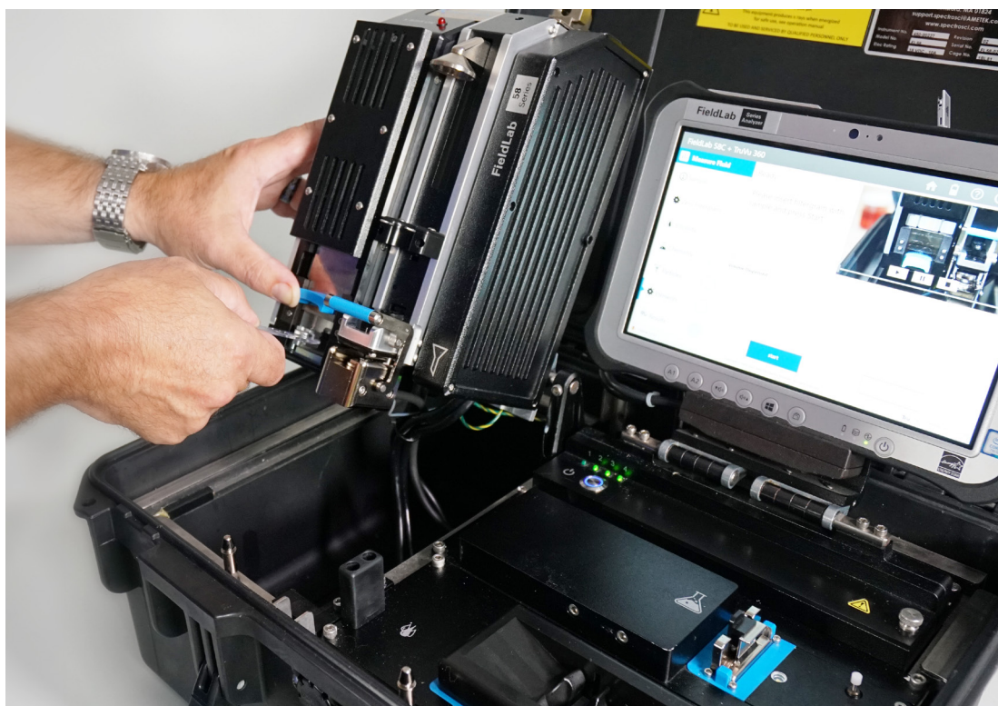
Figure 4: FieldLab 58 portable fluid analysis system reports kinematic viscosity, infrared chemistry and contamination, pore blockage particle count, and X-ray fluorescence multi-element large particle wear debris analysis.
