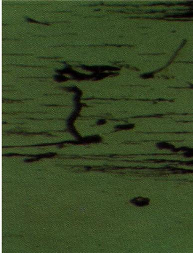
Figure 11, Ferrogram from Compressor Used Oil Sample
