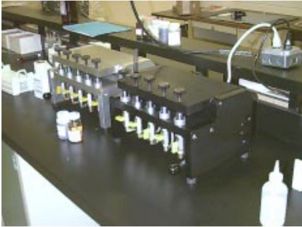
Figure 14, Multi-station RFS Sample Preparation Fixture
