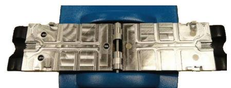
information, such as oxidation, nitration, sulfation, anti-wear additive, total base number, water, glycol contamination, and soot. The technology was recently granted an ASTM D7889 standard method.
