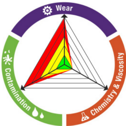
Figure 3. Trivector™ graphic for wear, contamination, chemistry alarm status
