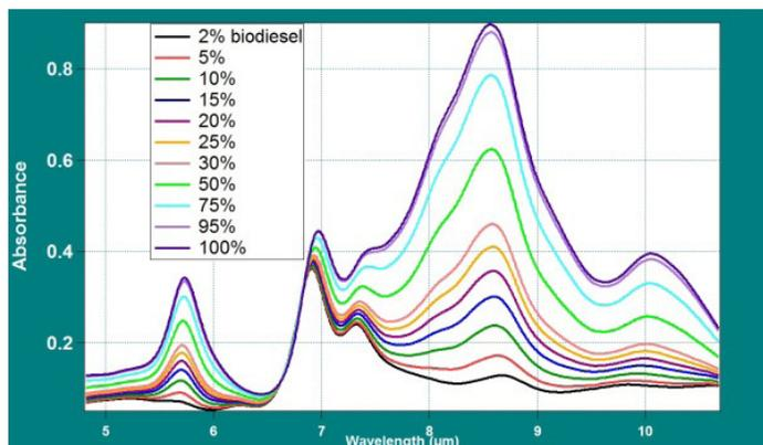
Figure 2: Spectra of different biodiesel concentrations
