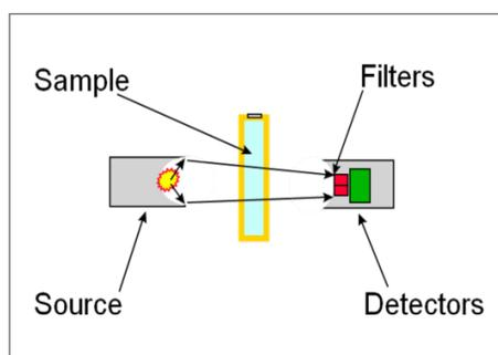
Figure 1: Schematic of a transmission sample system
