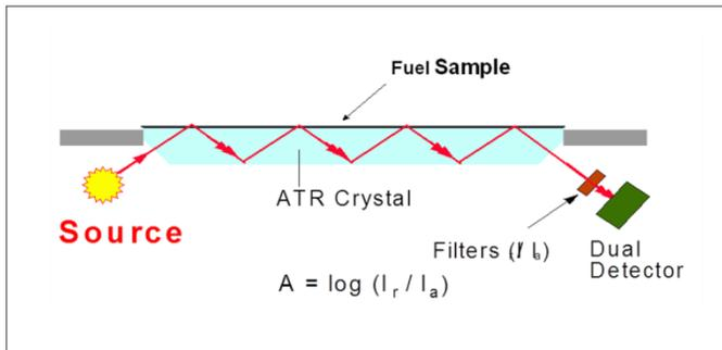
Figure 3: Schematic of an ATR sample stage
