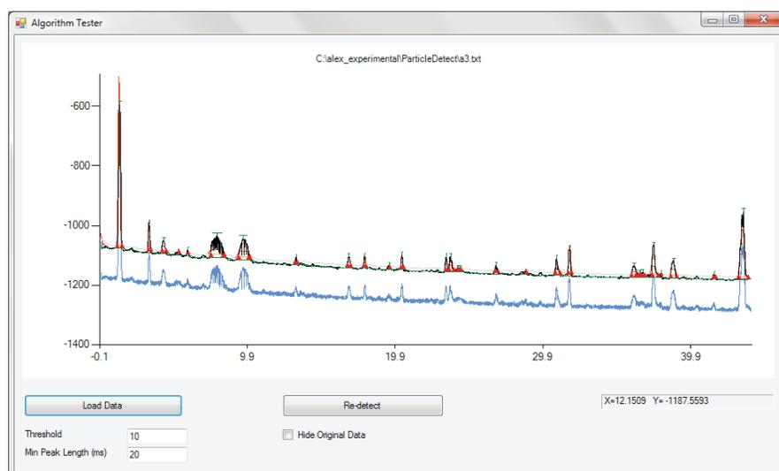
**Figure 1:** Example raw signal of individual magnetic particles passing through the Q230. The peaks in the data indicate that an individual magnetic particle has passed through the device. The red dots indicate the software's determination of the beginning and end of each peak. The hatches on the top of each peak indicate the Q230's determination of the height of each peak using its built-in peak detection algorithm.
