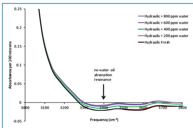
**Figure 3:** Infrared signature of emulsified and free water in oil: The presence of such contaminants is marked by elevated absorption across the infrared with no peak, a signature of the scattering of the infrared light by the water.
