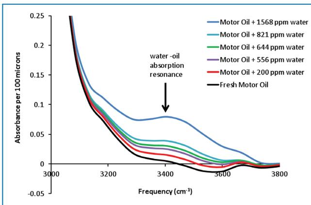
**Figure 1:** An example of dissolved water absorption in motor oil: FluidScan spectra depicting a series of motor oil samples with increasing amounts of water. The main absorption resonance is centered at 3400  $\text{cm}^{-1}$ .
