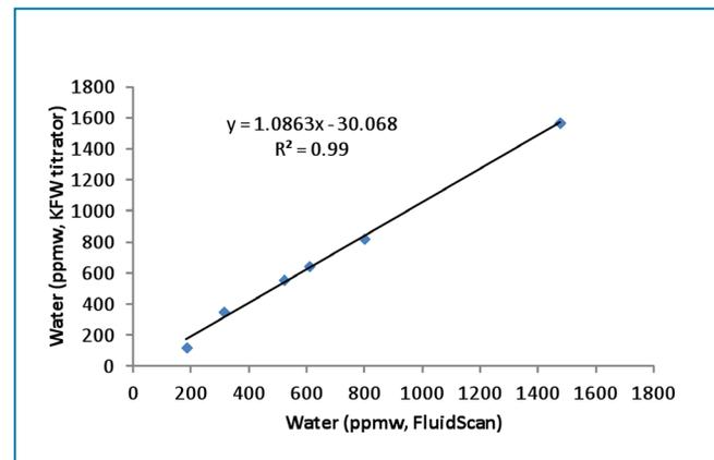
**Figure 2:** Comparison of FluidScan water readings from the analysis of the spectra in Figure 1 to ASTM D6304 Karl Fischer water titration.
