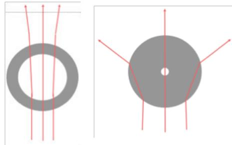
At left, laser light refracts only slightly because the refractive index of the water is very close to that of the oil. At right, laser light refracts considerably because the refractive index between the oil and the air differs greatly.
