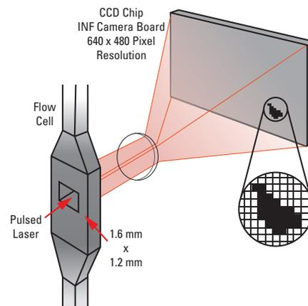
The laser illuminates the sample, and an optical lens magnifies the laser light. A CCD video camera captures the images of the sample and stores them in memory. These images are analyzed for size and shape. An equivalent circular diameter or ECD is calculated for each image and particle count and size distribution is reported along with ISO codes. The LNF provides other output formats but ISO 4406 is the most common.
