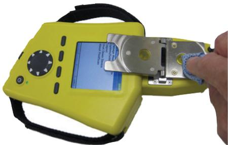
**Figure 2:** Patented flip top cell eliminates the need for solvents to clean.
